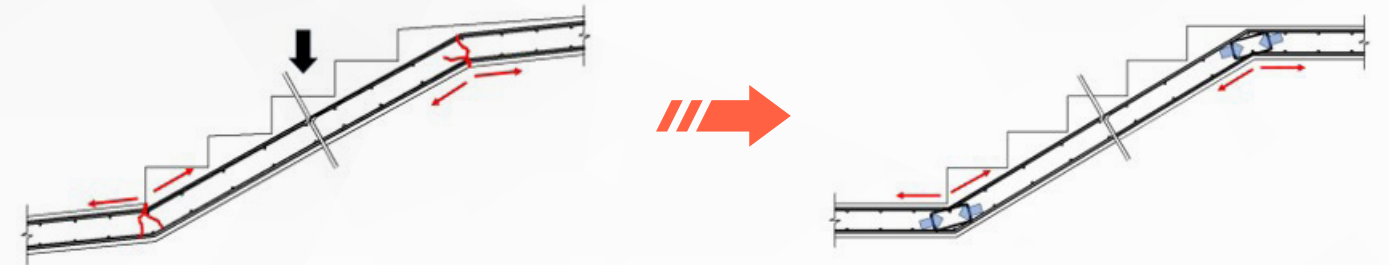
Tensile resistance of stair-bend reinforcement
